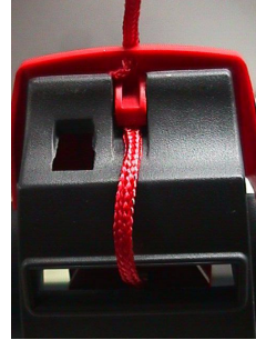
Photo 14. Improperly routed safety cord.
