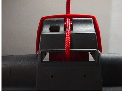
Photo 13. Properly routed safety cord.
